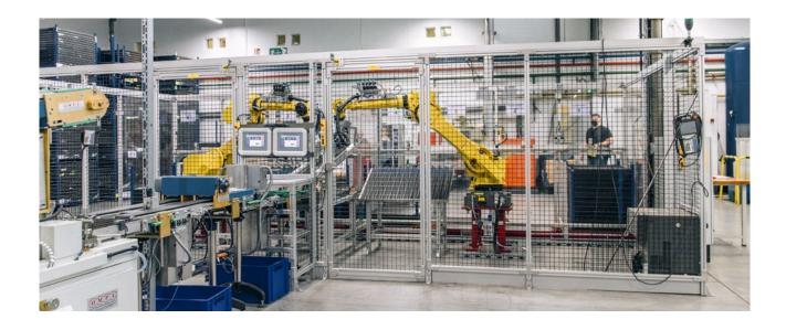
Securing two access doors to a system with robot and conveyor belt
