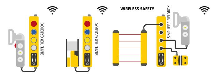
Whether CAN or wireless safety, all information reaches the Siemens controller via the Simplifier Gateway on PROFIsafe and can be programmed and managed centrally in the TIA programming software.
