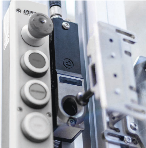
ATOM safety guard locking, connected to the wireless safety controller Safety Simplifier
