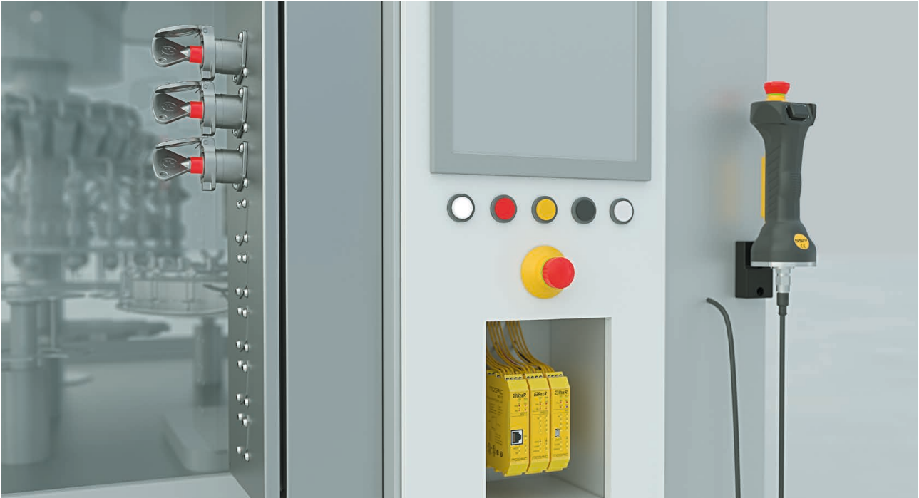
Safe speed monitoring with the MOSAIC safety controller, ZEUS enabling switch, EDI emergency stop button, Simplifier push-button elements
