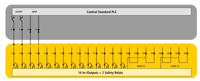
Hard-wired interface: Unsafe communication with only two inputs and outputs
