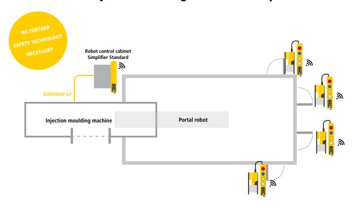
Example of an injection molding plant with Safety Simplifier
