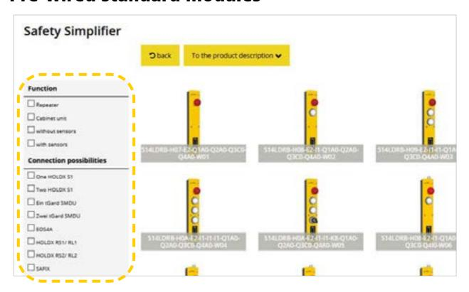
Plug & Play: The pre-wired Safety Simplifier standard variants can be directly connected and used. With the help of pre-configured connection options for safety solutions, such as safety switches or curtains, a plant can be put into operation in the shortest possible time without any wiring effort.
