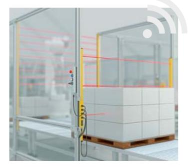
Safety Simplifier interlocking function with EOS4 light grids for unloading of pallets
