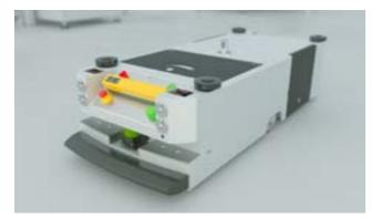
With the Safety Simplifier, automated guided vehicles can be switched off safely and wirelessly. Safe networking to production plants is possible at any time.
