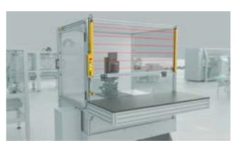
The communication does not necessarily have to be wireless. The Safety Simplifier can also be used as a stand-alone solution for small systems and does not require space in the control cabinet.
