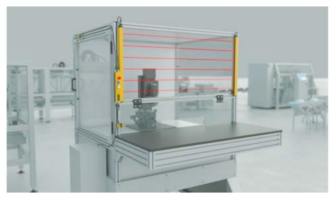
Safety controller directly integrated in the operational unit, without additional safety controller in the control cabinet
