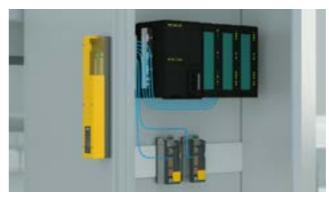
External mounting on the control cabinet saves space. Thanks to the LED display, diagnosis can be done without opening the control cabinet.
