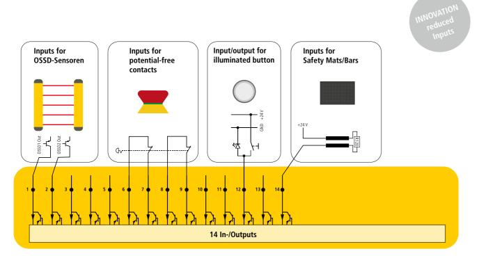
Connection example, safe inputs to the Safety Simplifier S14
