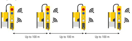
With the Safety Simplifier, very large ranges can be realized. The range between two participants is up to 100 meters. The integrated repeater function effectively extends the range. Safety Simplifier repeater modules can also be integrated to increase the range or to optimize the mesh network.
