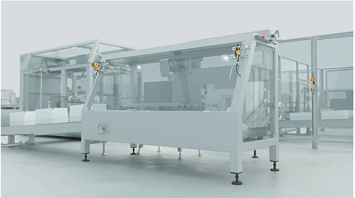
Case erector with process guard locking HOLDX RS1
