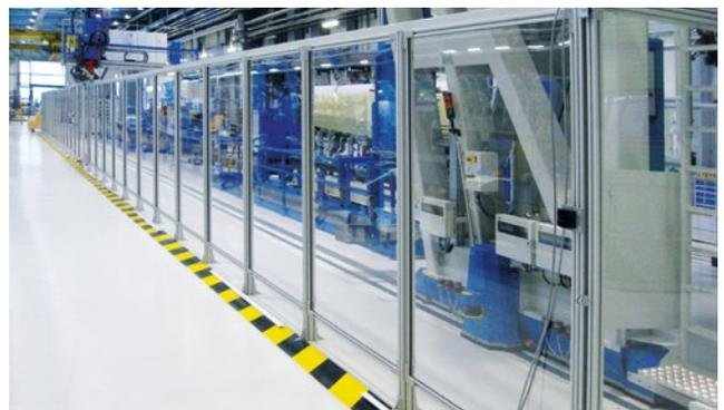
Thanks to polycarbonate fillings, the machines stay perfectly visible and provide not only grip guard and protection, but also good-looking machine safety.
