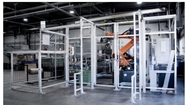
The route of the fence follows the route of the machine and the application. Angles, slopes, fillings and much more can be customized with the Flex-Line model.
