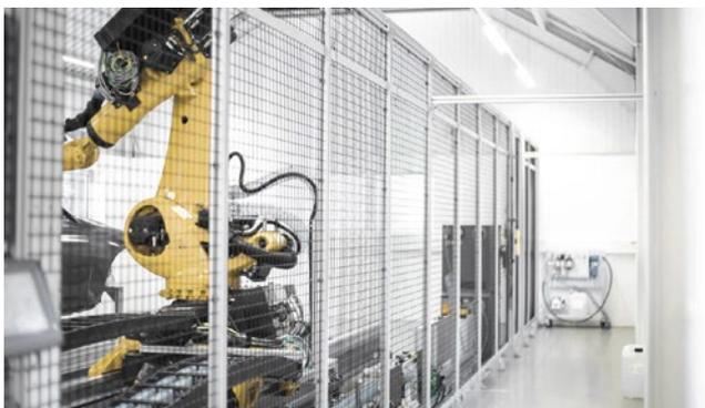
Stable spot welding grid with reinforcing fixation technology and robust aluminum profiles. SSP safety fences are regularly tested using pendulum and ballistic tests.
