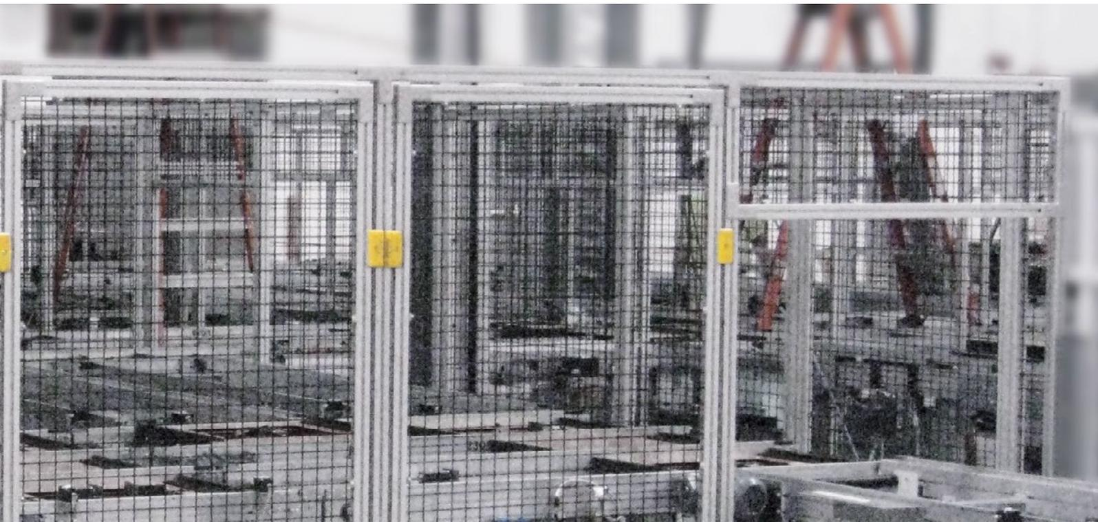
The quick-release panel is a real improvement during maintenance work. Using the supplied special key, one person alone is able to open and remove the quick-release panel, if necessary.
