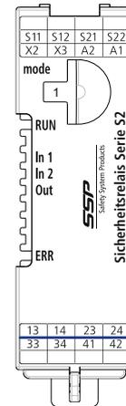
Against all other connection terminals, the safety contacts 13-14 and 23-24 comply without additional measures with the requirements for double insulation in accordance with IEC/EN 60664-1 and are to be used with switch voltages > 50 V. The safety contacts 33-34 comply with the requirements for basic insulation.
