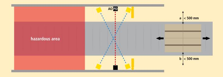
• If there is a risk of body parts being crushed between the load and stationary parts, DIN EN 349:2008 recommends a minimum distance of 500 mm between the moving load and the stationary parts of the system to avoid the risk of crushing or shearing. Further details are given in EN 349.
