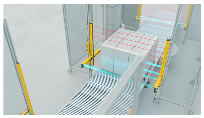
T-Muting with M5 multi-beam sensors for complex charges and partial muting
