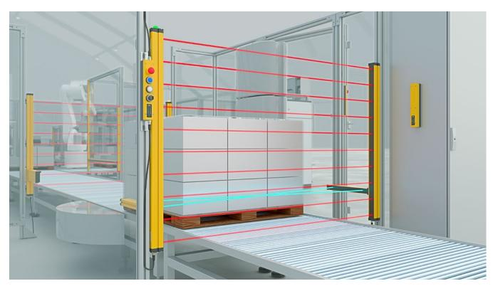
L-muting for unloading of pallets with crossed muting sensors
