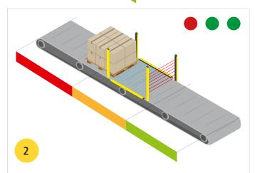
The pallet has passed and switched off the first light grid. There is no person inside the lock. The horizontal light grid ③ and the light grid outside ② are active.
