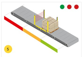
The pallet occupies the horizontal 3 and the outer 2 light grid. The inner light grid 1 protects the system against intervention.
