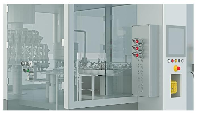
MOSAIC safety controller and mGard key transfer system with removal unit
