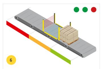
The pallet only occupies the outer light grid ②. The horizontal light grid ③ is active. There is no one inside the lock.
