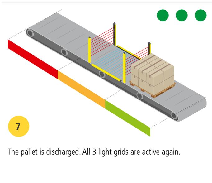
If malfunctions occur during the lock function (e.g. unauthorized access by persons to the lock), the override function makes it possible to manually discharge the pallet on site and restart the system.
