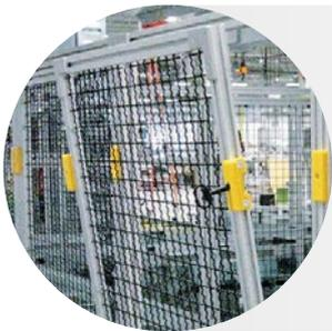
Fast removal fields reduce maintenance times with infrequent access. Thanks to the special key, no electronic protection is required.
