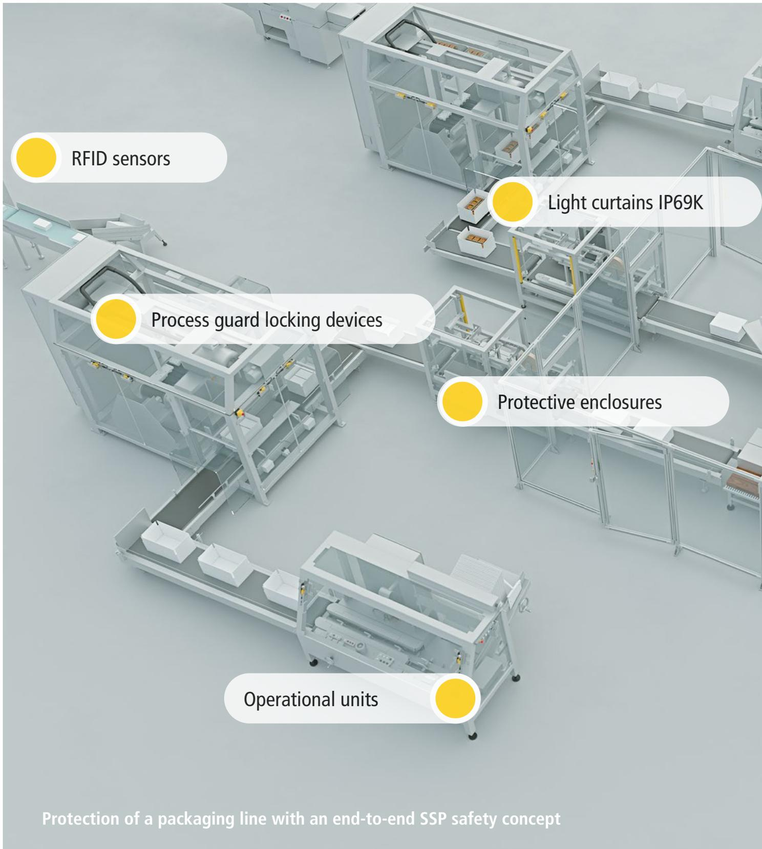
Protection of a packaging line with an end-to-end SSP safety concept
