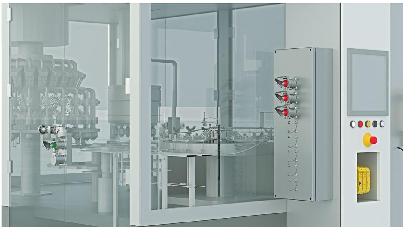
MOSAIC safety controller and mGard key transfer system with removal unit
