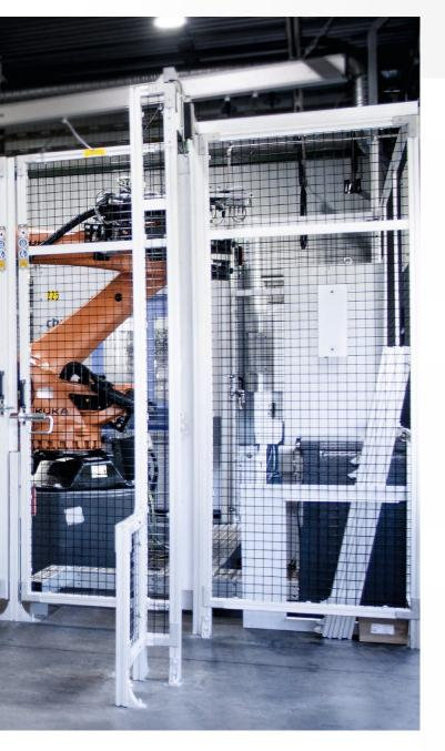
The combination of floor attachment bracket and aluminum profile easily compensates for any unevenness.
