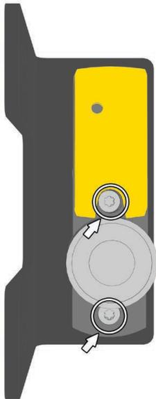
Fig. 7: Attach the process lock to the mounting plate and tighten the Torx screws M6 x 25 mm.
