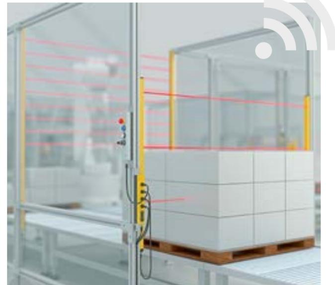
Safety Simplifier interlocking function with EOS4 light grids for unloading of pallets
